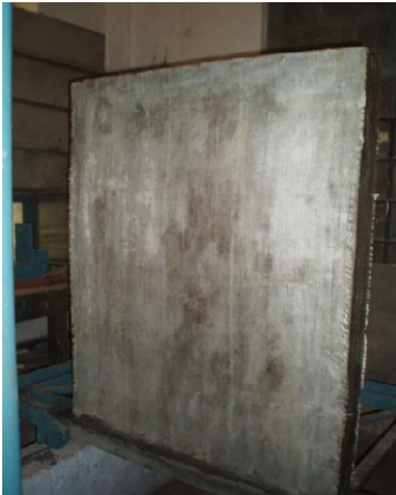
Figure 4. GFRP wrapped wall
