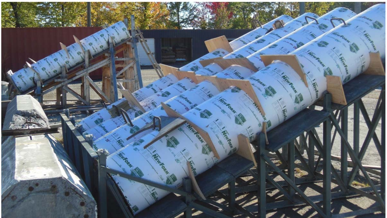
Figure 5. The B.P GFRP cages inside Sonatubes.
