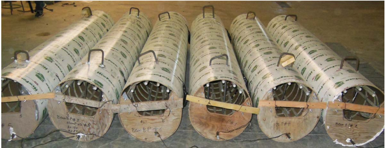
Figure 5. The B.P GFRP cages inside Sonatubes.
