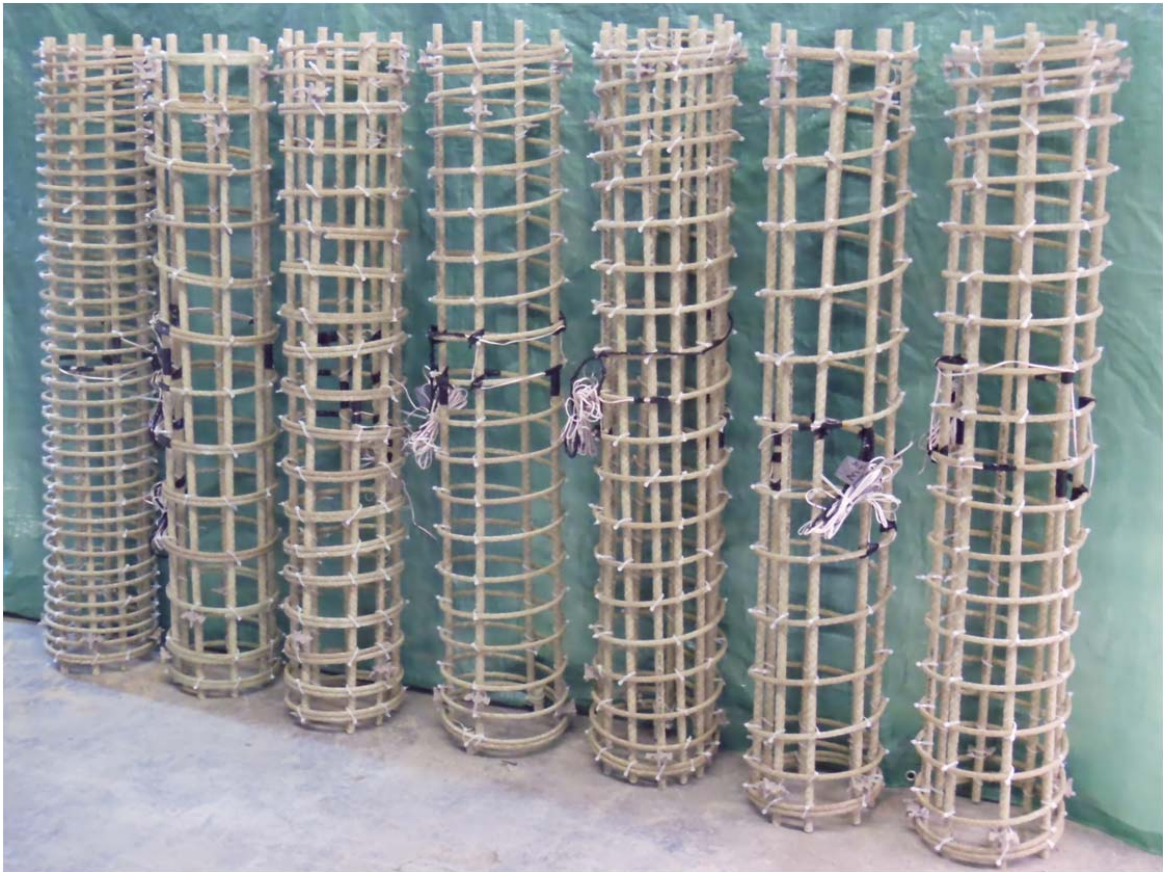
Figure 11. Overview for B.P GFRP cages
