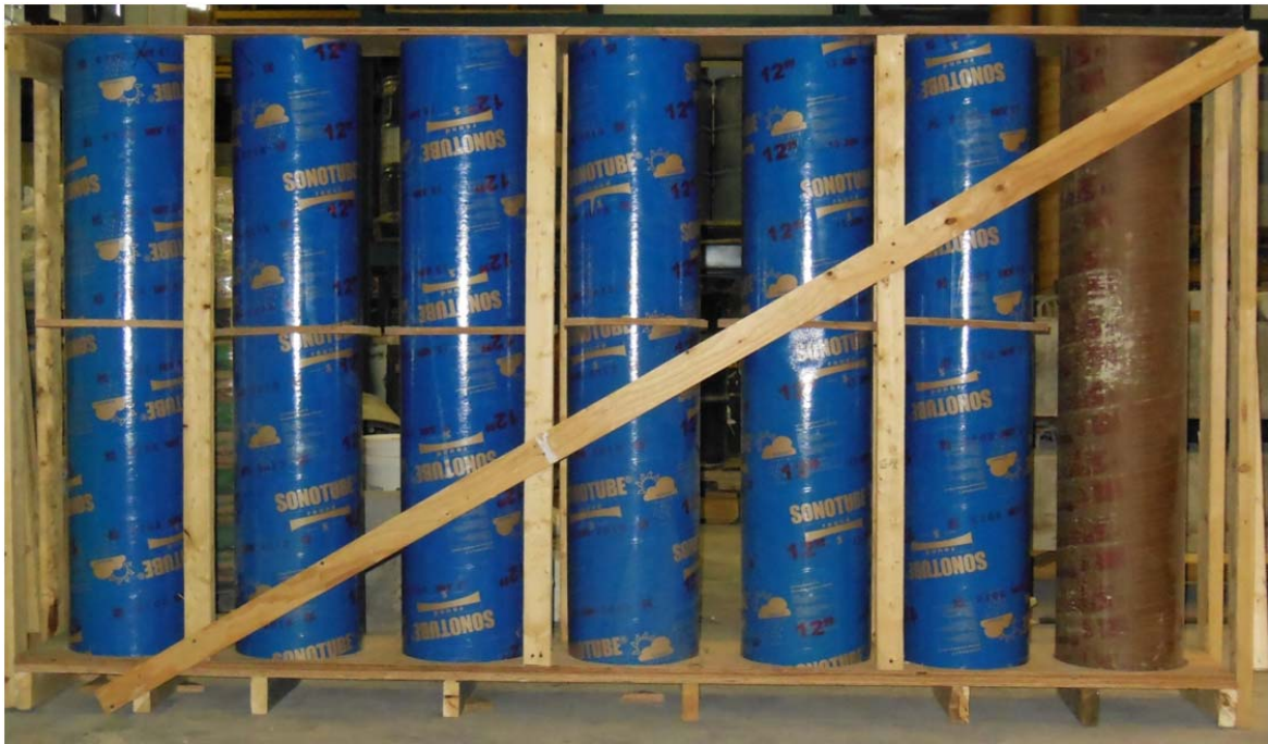
Figure 12. Overview of the columns formwork
