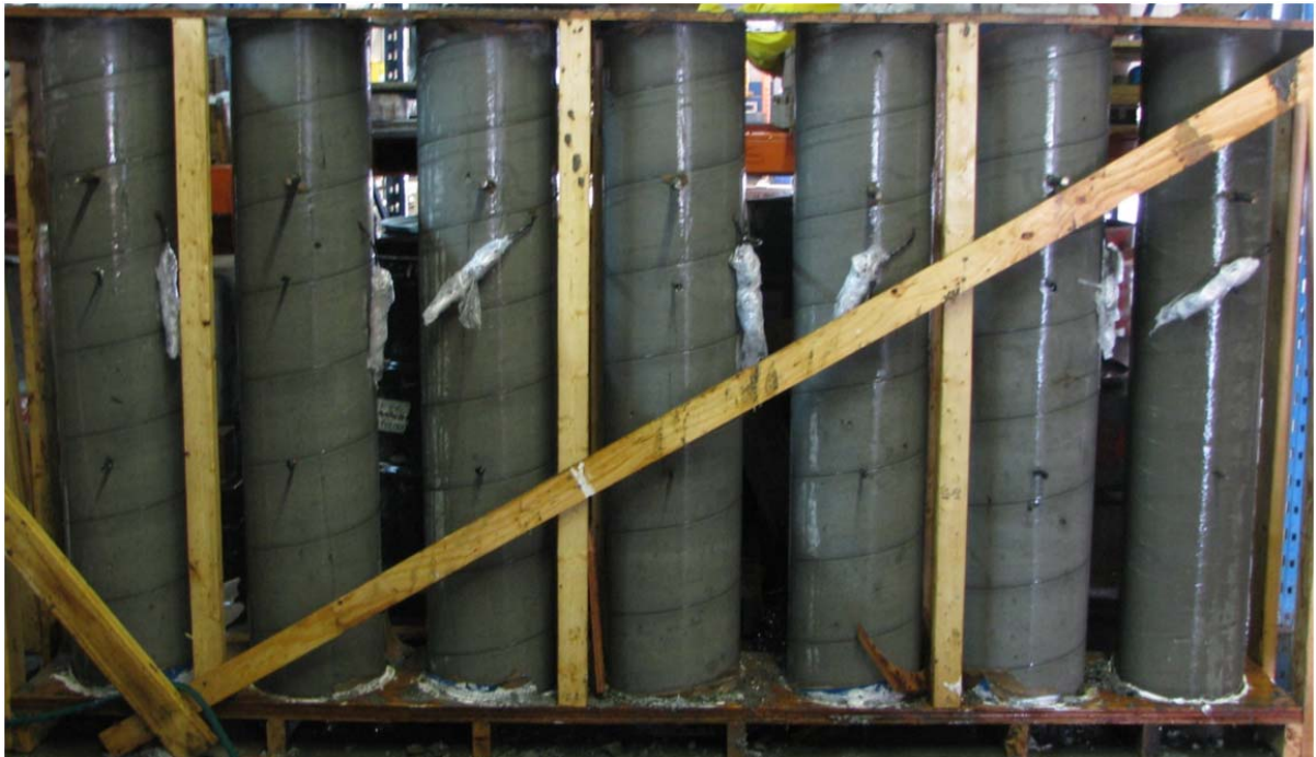
Figure 15. The columns after casting
