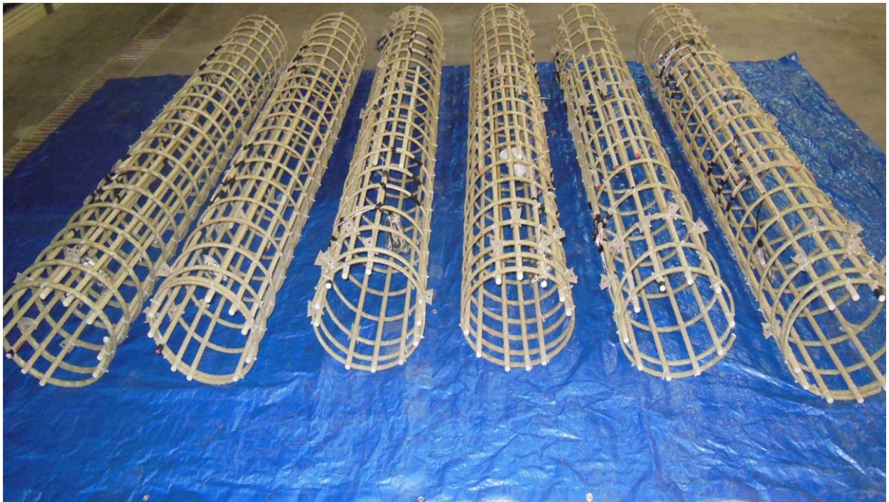
Figure 4. Overview for the B.P GFRP cages with strain gages.
