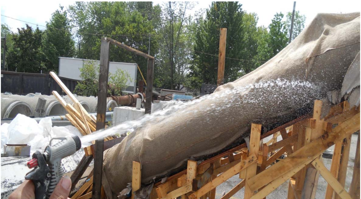
Figure 8. Curing of circular specimens
