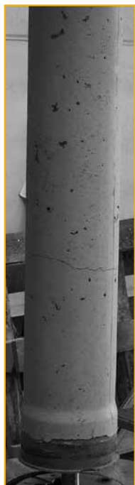
first crack (150 N/mm 2 )
