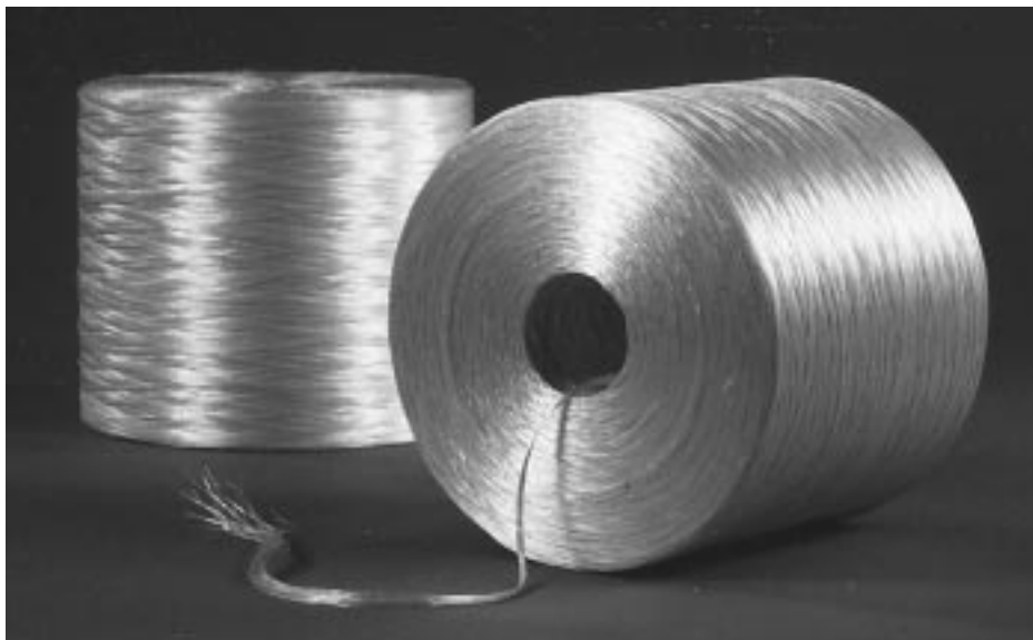
Fig. 2.6—Glass fiber rovings [Owens-Corning Fiberglass Corporation (1995)]
