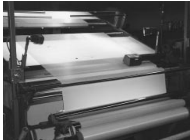
Fig. 2.9—Glass fiber cloth during weaving and inspection [Clark-Schwebel, Inc. (1995)]
